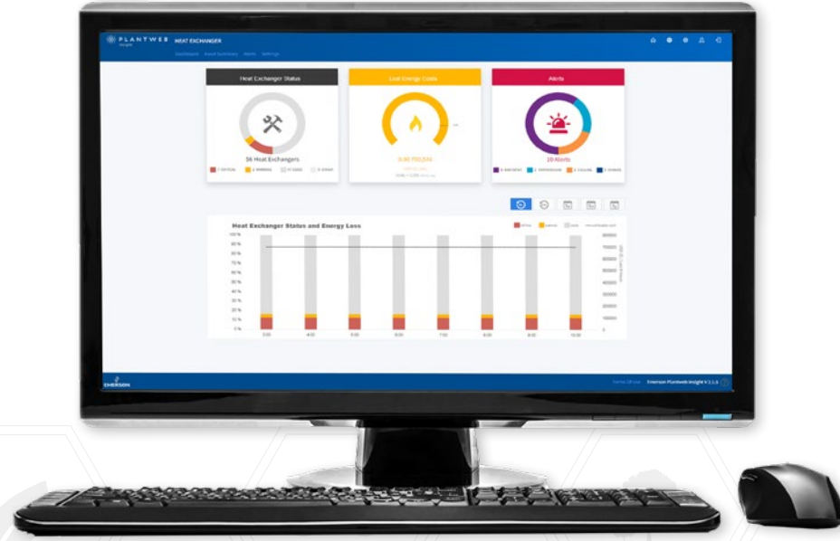
Figure 13: A Plantweb Insight dashboard designed for heat exchangers monitors operational changes that indicate the first signs of fouling or internal leaking, along with other efficiency indicators.
