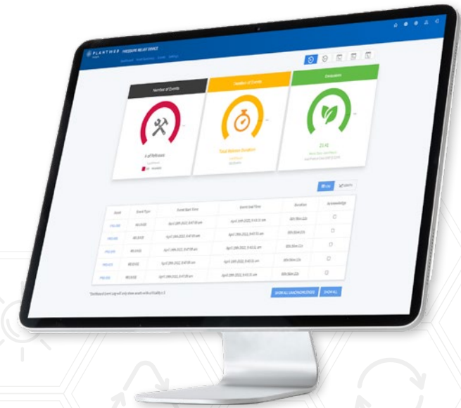
Figure 7: A Plantweb Insight dashboard designed for PRVs times releases, and it also alerts the maintenance team if the valve does not close completely after a release.
