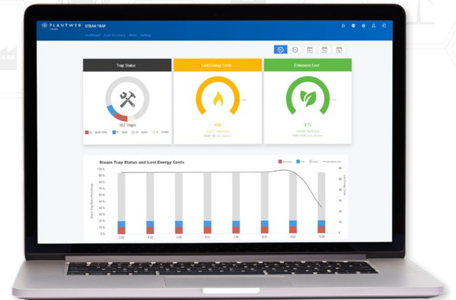
Figure 5: A Plantweb Insight dashboard designed for steam traps alerts the maintenance team as to which are working correctly, and which are inoperative.
