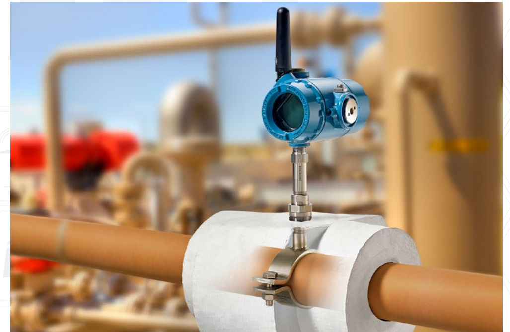
Figure 12: Emerson's Rosemount X-well™ technology reads the temperature inside a pipe without the need for a penetration. It sends data via WirelessHART.
