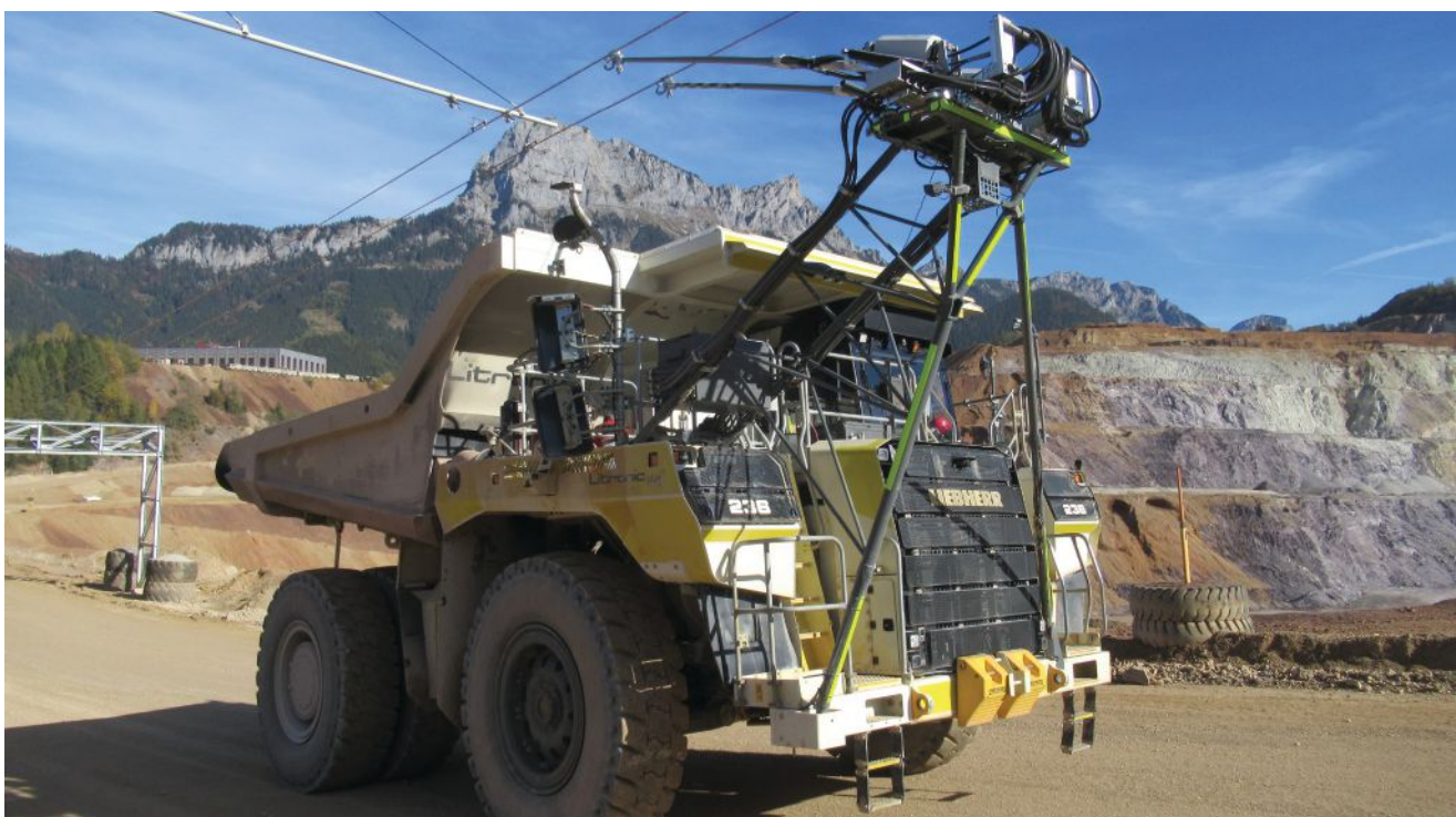
Liebherr offers trolley assist systems for most of its haul trucks. (Photo: Liebherr)
