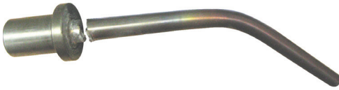
Figure 3-91 – Example of a Thermowell Failure
