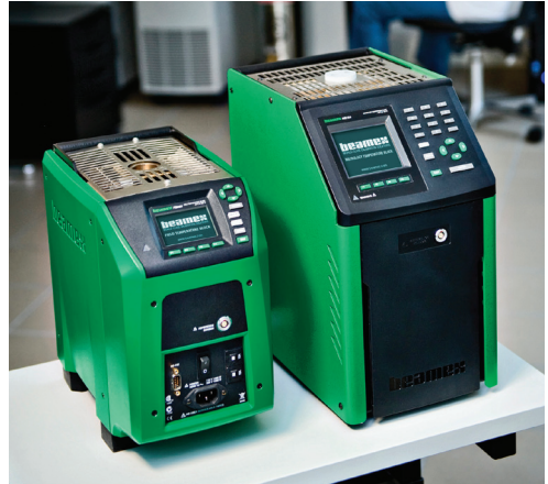
Figure 5-7 – Typical Field Dry Block and Metrology Grade Dry Blocks (Courtesy of Beamex)
