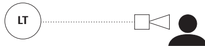
Figure 3.6: Manual overfill prevention systems (MOPSs) usually consist of a level transmitter (LT) connected to an audiovisual alarm that notifies an operator to take the appropriate action, e.g. closing a valve
