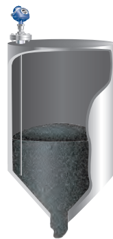
Figure 4.35.1: Powder level with guided wave radar
