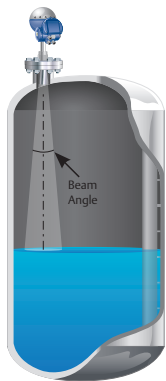
Figure 6.6.3: Beam width angle for the Rosemount 5600
