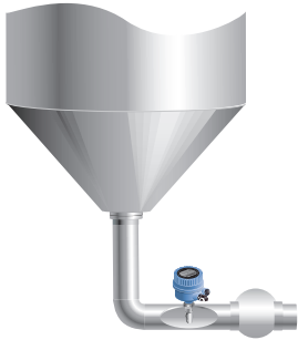
Figure 9.1.4: Pump protection or empty pipe detection
