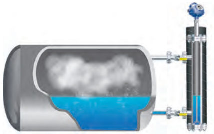
Figure 4.22.1: Measuring level on refrigerants with guided wave radar
