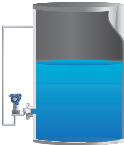
Figure 7.1.1: Illustration of a wet leg installation
