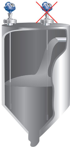
Figure 5.9.2: Mounting position in solids
