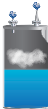
Figure 4.29.1: Ammonia (aqueous) level with non-contacting radar
