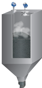
Figure 4.33.2: Bottom ash with guided wave radar or non-contacting
