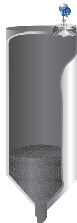
Figure 4.26.1: Coal bunker level with non-contacting radar
