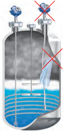
Figure 5.9.1: Mounting position in liquids
