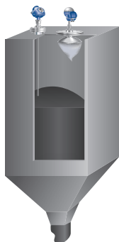
Figure 4.33.1: Ash hopper or fly ash with guided wave radar or non-contacting
