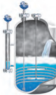
Figure 2.1.1 GWR can handle disturbing objects and tough process conditions. It can be installed directly in the tank or in a by-pass chamber
