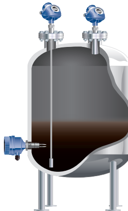
Figure 4.13.1: Hydraulic oil tanks with guided wave radar, non-contacting radar and vibrating fork switch.
