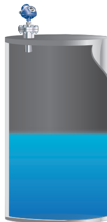
Figure 4.19.1: Water and boric acid storage with a non-contacting radar
