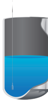
Figure 7.6.1: 9710 cable suspended mounting configuration
