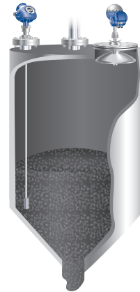
Figure 4.17.1: Rock salt level with non-contacting or guided wave radar
