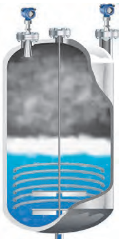
Figure 4.9.1: Reactor vessel level with non-contacting radar
