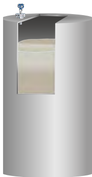
Figure 5.2.10: Slacked lime powder silo with non-contacting radar device
