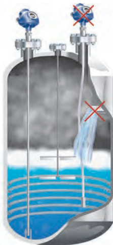
Figure 6.10.1: Mounting position in liquids
