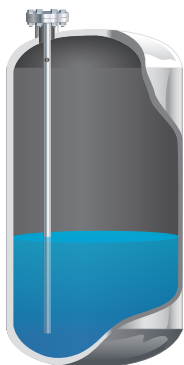
Figure 6.13.8: GWR measuring level in stilling well
