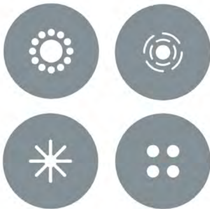
Figure 7.15: A few examples of multi-hole orifice plates.
