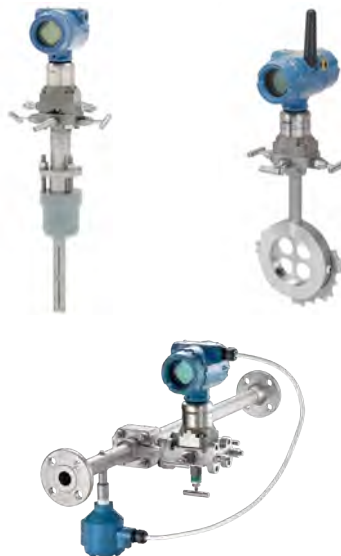
Figure 8.13: Flow meter assemblies using the same transmitter. Many flow meter configurations are possible due to the wide range of available primary elements. Clockwise from top left: Rosemount 3051SFA Annubar, Rosemount 3051SFC Compact Conditioning Orifice, and Rosemount 3051SFP Integral Orifice Flow Meter.
