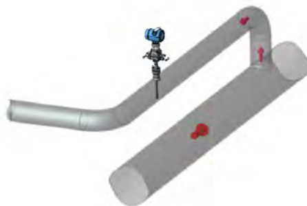
Figure 10.19: A piping branch and flow meter located.
