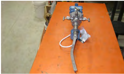
Figure 10.1: Rosemount 485 Annubar Primary Element damaged by improper installation.
