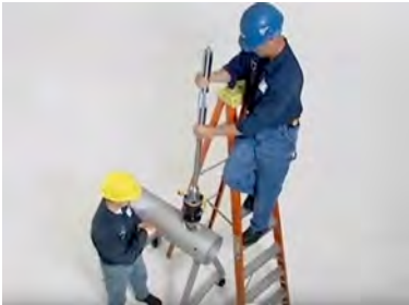
Figure 10.36: A simple hand-operated hot tapping machine.
