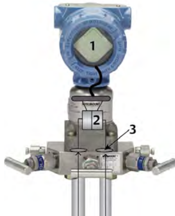
Figure 8.2: The pathway of a physical pressure measurement is converted into an electrical signal.
