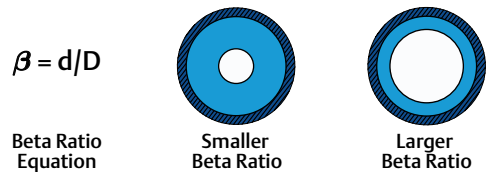
Figure 2.15: Area meter beta ratio.
