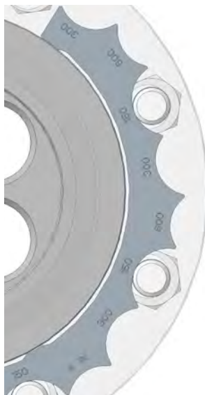
Figure 9.17: Rosemount 405 platform alignment ring.
