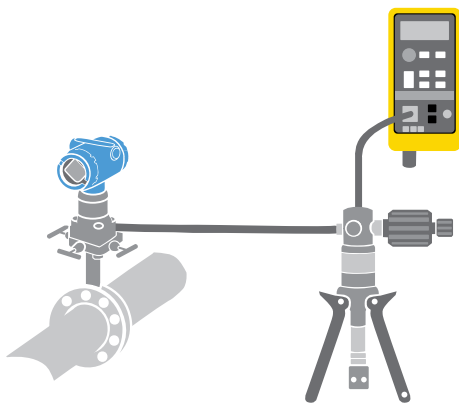
Figure 11.10: A reference pressure source connected to a transmitter.
