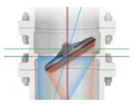
A non-rubbing design and zero cavities for solids accumulation eliminates the need for planned maintenance in most applications. For mandatory maintenance, simple, interchangeable spares are available at a lower cost compared to gate valves.
