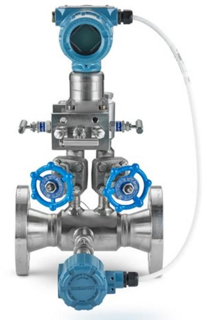
Figure 4.6: To cover a flow turndown range of 100:1 with the degree of accuracy required, one flow meter can't do the job, so two must operate in parallel on low- and high-steam lines. Valves direct the flow appropriately.
