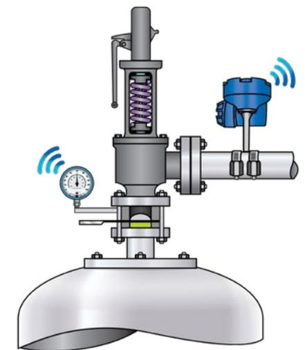
*Figure 4.4: Mounting a Rosemount 708 Wireless Acoustic instrument on the discharge pipe of a PRV detects when release incidents happen, and if leakage continues due to an incomplete seal. No process penetration or shutdown is necessary for mounting.*
