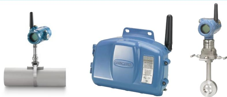
Figure 2.3: Using WirelessHART instruments for heat exchangers simplifies installation. Rosemount X-well™ Technology (left) does not require a thermowell or process penetration. Where conventional temperature sensors are preferred, the Rosemount 848T Wireless Temperature Transmitter (middle) can send data from four sensors via one signal. A Rosemount 3051SFC Wireless Compact Orifice Plate Flow Meter (right) can measure fluid flow in tight spaces.
