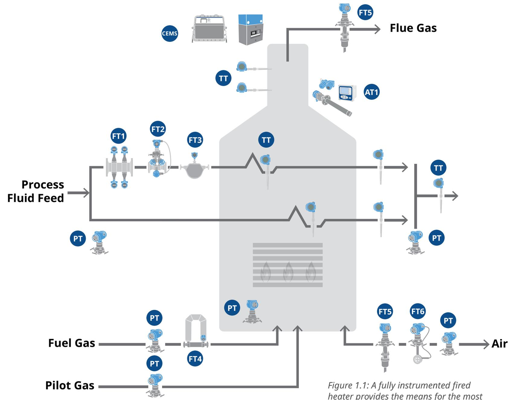
Figure 1.1: A fully instrumented fired heater provides the means for the most sophisticated control, ensuring maximum efficiency with the lowest emissions.
