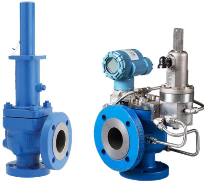
Figure 4.3: Direct spring load (left) and pilot-operated valves (right) function differently, but both can leak, making characteristic sounds. Pilot-operated valves can also be diagnosed by monitoring internal pressures.
