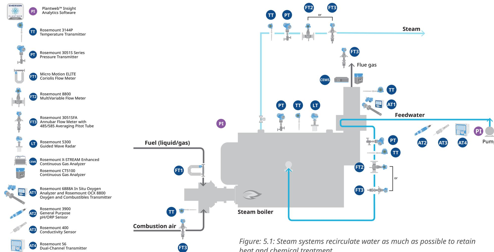
Figure 5.1: Steam systems recirculate water as much as possible to retain heat and chemical treatment.
